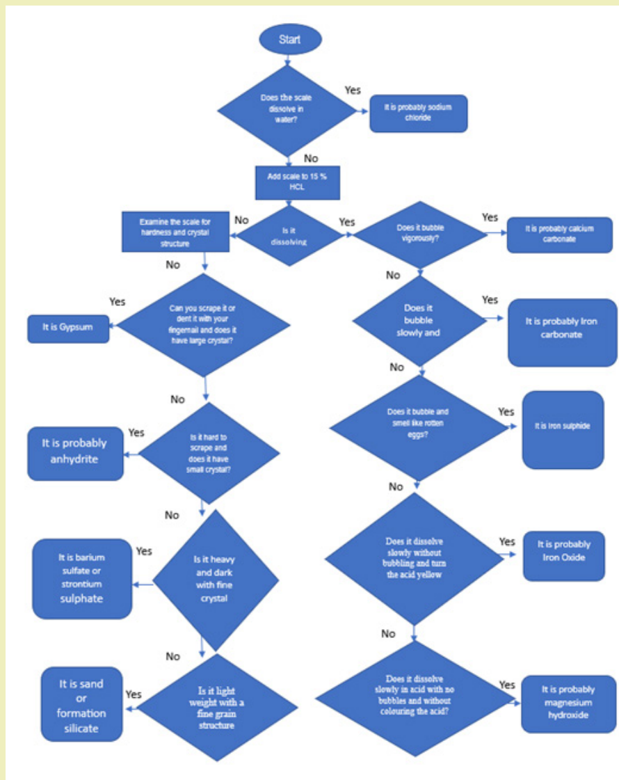
Figure 2: Flowchart for field identification of scale
