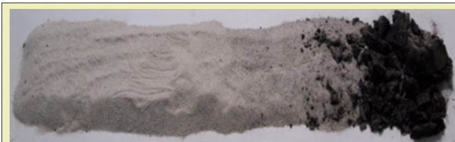
Figure 9: Color of sand after fire flooding experiment.
