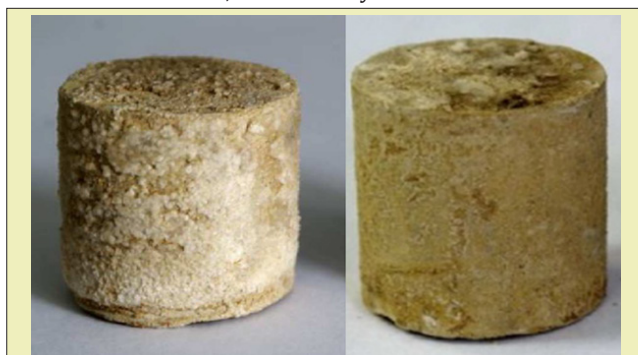
Figure 1: Samples of cement stone based on PCT-1-50 and high alumina cement.
